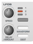
As with an Envelope, the waveforms generated by the LFOs may be fed to other parts of the synthesizer to create the desired movements in the sound.
