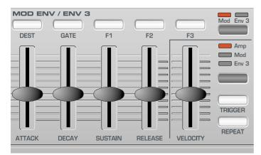
The MOD Envelope may be used to control other sound elements of the synthesizer throughout the duration of the sound. It can control Oscillator Pulse Width, Filter frequency and Oscillator Pitch.
