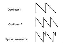
It can be seen that the resulting synced waveform has subsequently been modified into a different shape. Altering a waveform's shape in this way introduces new harmonics into the sound which gives the resulting waveform its distinctive synced sound qualities.
