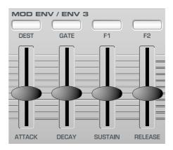
A third Envelope Generator called Envelope 3 is also used by the KS Synth for specialised purposes (such as FM control). Unlike the other two main Envelope Generators, this Envelope only has Attack and Decay phases.
