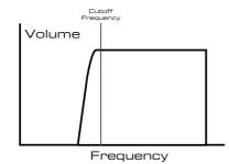
When the Band Pass Filter is used, only a narrow band of frequencies centered on the cutoff frequency point are let through. All frequencies outside this band are removed. It is not possible to fully open this type of Filter, allowing all frequencies to pass through.
