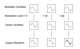
In the illustration, the Oscillators are producing Sine waves. It is the *change* in harmonics over time that makes a sound interesting to our ears.
