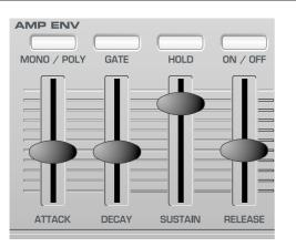
The Envelopes are used to shape a sound throughout its duration. The AMP Envelope always determines the volume of the sound with respect to its duration.
