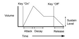
When controlling Volume, these controls adjust the following phases of the Envelope as shown in the illustration.
