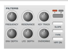
The Filter can be used as a Low Pass, High Pass or Band Pass type.
