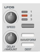
There are two LFOs - Low Frequency Oscillators - available on the KS Synth. These produce regular electronic variations which are too low to be heard when converted into audio vibrations. They can modify various elements of the sound, producing regular changes in pitch (vibrato), pulse width or filter Cut off.
