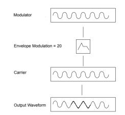
It can be seen that the output waveform begins by being identical to the carrier, but becomes more complex (harmonics are added) as the amount of FM modulation increases via the envelope. It then returns to a simple wave again as the envelope decays.
