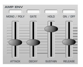
Each envelope generator has four slider controls which are used to adjust the shape of the envelope.
